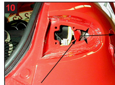
10 Rear wing: Remove tail light. Treat via existing holes.
