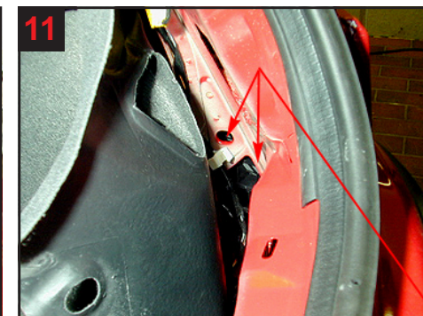
11 Rear wing from boot: Flip up lining for treatment of bottom in rear wing.
