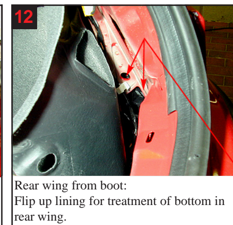
12 Rear wing from boot: Flip up lining for treatment of bottom in rear wing.
