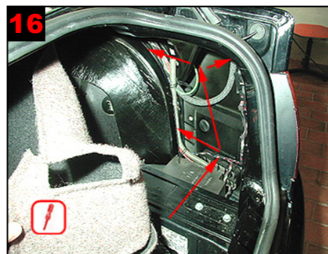
16 Rear wing: Flip felt, treat in all directions and right across wheel arch.
