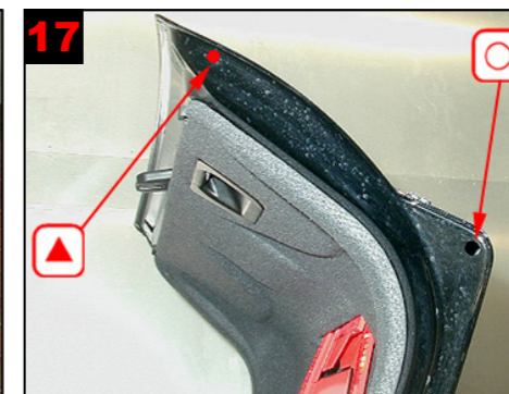
17 Tailgate side: Treat via 1 drilled hole and existing hole.
