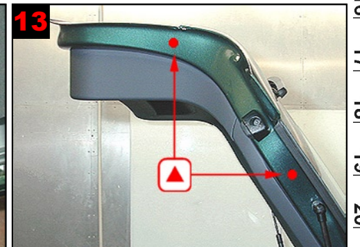
Tailgate side: Drill 2 holes for correct treatment.
