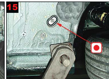
15 Small cross member after front wheel arch: Treat via existing plugged hole.
