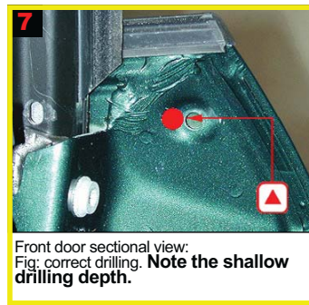
7 Front door sectional view: Fig: correct drilling. Note the shallow drilling depth.
