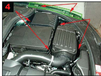
4 Front wing/wheel arch liner: Treat via existing holes and gaps.
