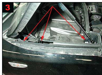
3 Engine compartment - sectional view: Treatment via existing gap by hinges for bonnet lid.
