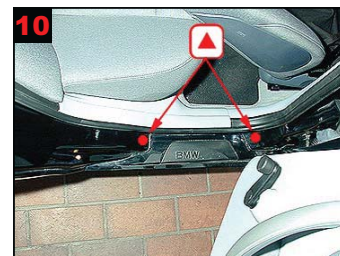
10 C-pillar/panel: Drill 2 holes for correct treatment.
