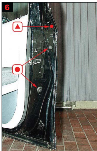
6 Front door: Door - top member. Treat via 1 drilled hole. Remainder via existing plugged holes.
