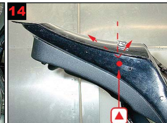
14 Tailgate side: Treat via 1 drilled hole each side. Treat with lance.
