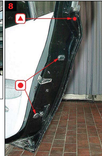
8 Rear door: Door - top member. Treat via 1 drilled hole. Remainder via existing plugged holes.
