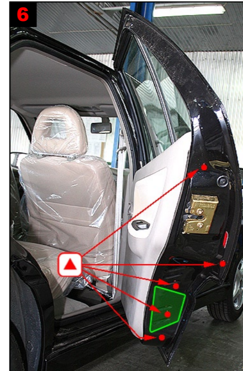
6 Rear door: Treat via 5 drilled holes.
