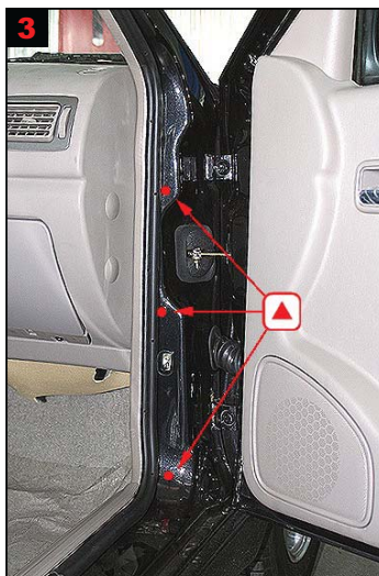
3 A-pillar: Treat via 3 drilled holes.
