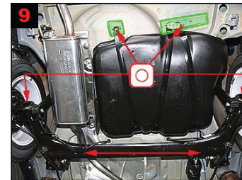
9 Rear axle assembly and reinforcements after tank. Treat via existing holes.
