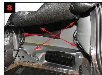
8 Rear wing: Treatment from boot. Flip up lining - treat in all directions.
