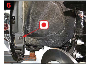
6 Wheel arch front, panel: Treat via existing plugged hole.
