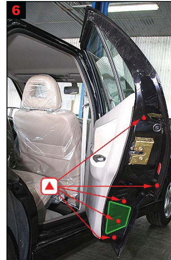
6 Rear door: Treat via 5 drilled holes.
