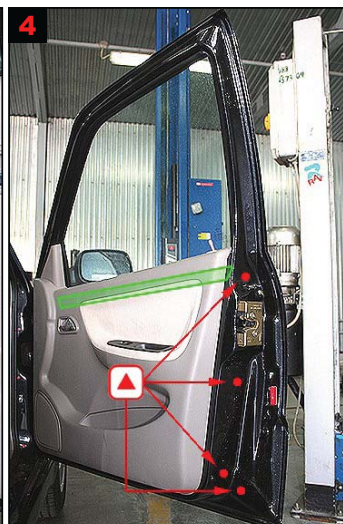
4 Front door: Treatment via 4 drilled holes. Lower drill hole is drilled with caution.
