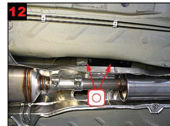
12 Reinforcement above silencer: Treat via existing holes and gaps.
