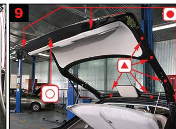
9 Tailgate: Treat via existing hole. Drill 5 holes and use 3 existing plugged holes.
