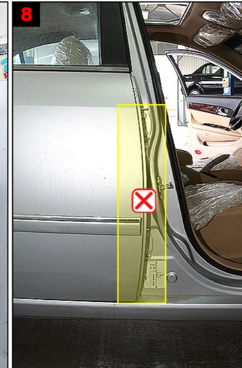
8 B-pillar: No treatment because of safety belt and airbag sensor
