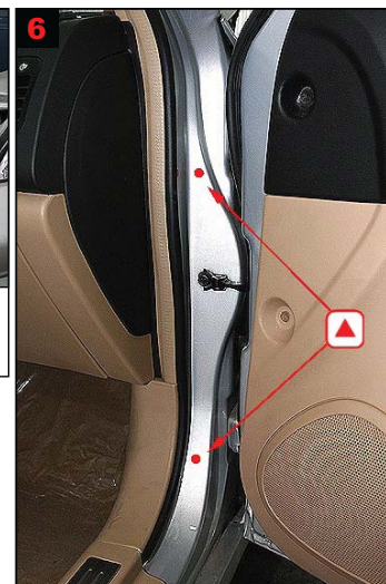
6 A-pillar: Treat via 2 drilled holes.
