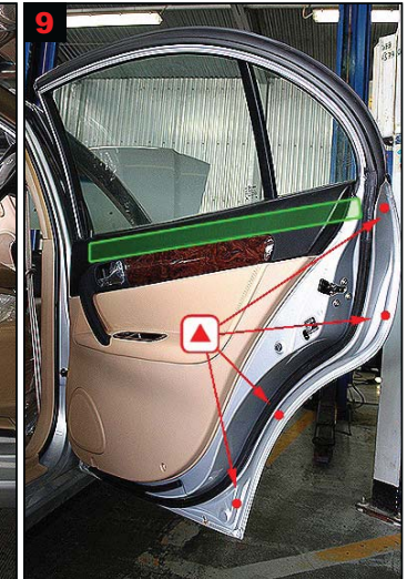
9 Rear door: Treatment via 4 drilled holes. Uppermost drill hole for inside reinforcement.
