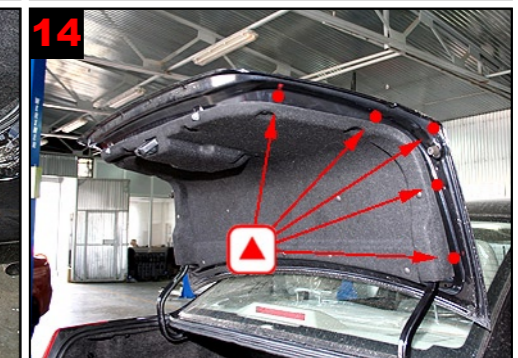
14 Tailgate: Treat via 5 drilled holes.
