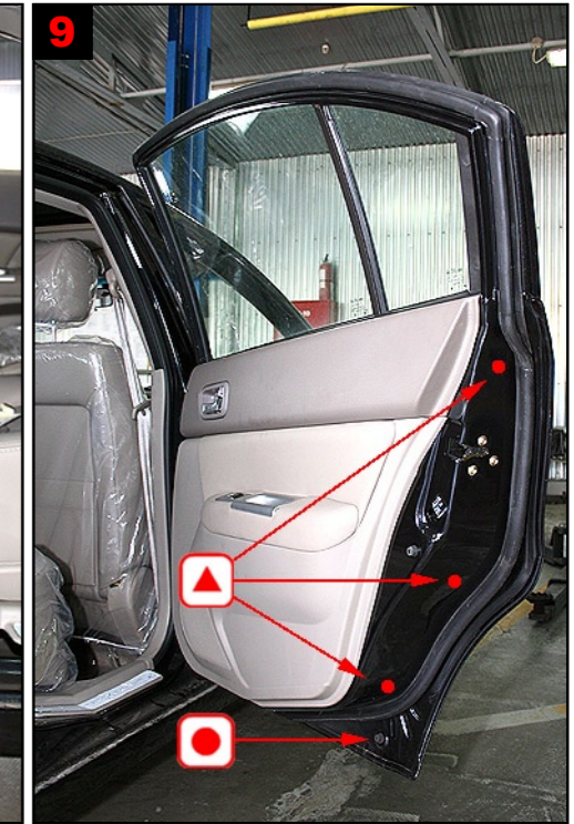
9 Rear door: Treat via 3 drilled holes and existing plugged hole.
