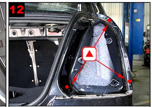
12 Rear wing and reinforcement: Treat via 3 drilled holes. No spraying towards cabin.
