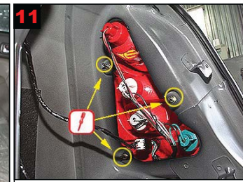
11 Removal of tail light from boot: Remove 3 nuts and pulling back.
