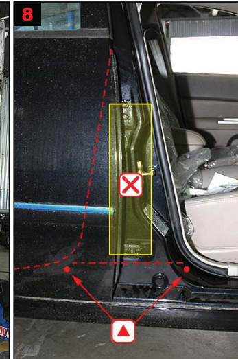
8 B-pillar: Treat via 2 drilled holes. No treatment upwards because of safety belt.
