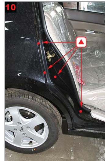
10 C-pillar: Treatment via 4 drilled holes. No spraying towards cabin.
