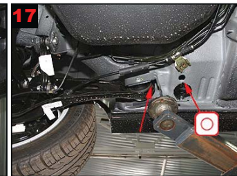
17 Longitudinal member before wheel arch rear and reinforcement: Treat via existing holes and gaps.
