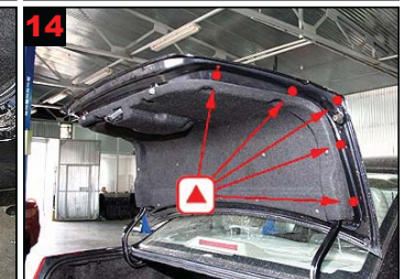
14 Tailgate: Treat via 5 drilled holes.
