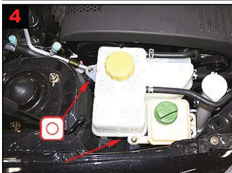
4 Engine compartment - sectional view: Reinforcement on spring strut right side. Treat via existing hole.
