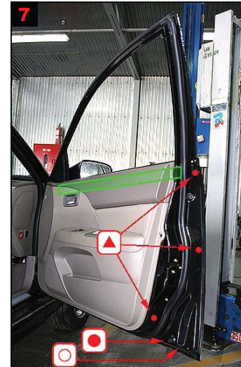
7 Front door: Treat via 3 drilled holes, 1 existing hole and 1 existing plugged hole. Uppermost drill hole for inside reinforcement.
