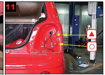
11 Rear wing: Treat via 1 drilled hole and existing hole.
