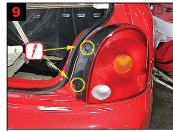
9 Removal of tail light: Remove 2 screws.
