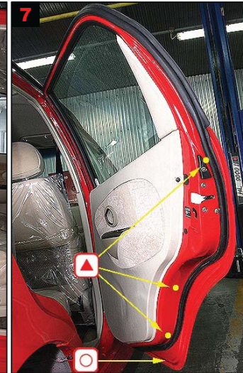
7 Rear door: Treat via 3 drilled holes and drain hole.
