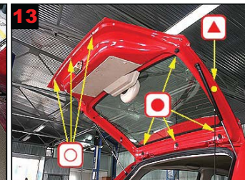
13 Tailgate: Treat via 1 drilled hole, 4 existing plugged holes and 3 existing holes.
