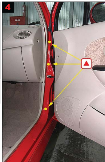
4 A-pillar: Treat via 3 drilled holes.
