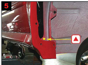
5 Wheel arch front/panel: Treat via 1 drilled hole.
