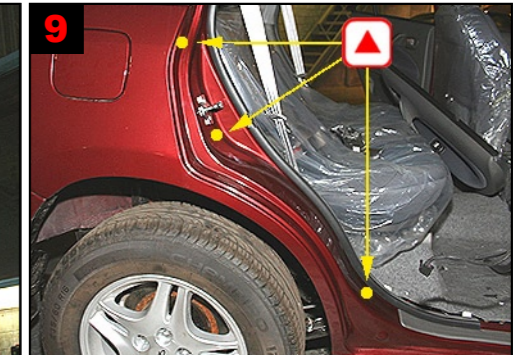
9 C-pillar: Treat via 3 drilled holes.
