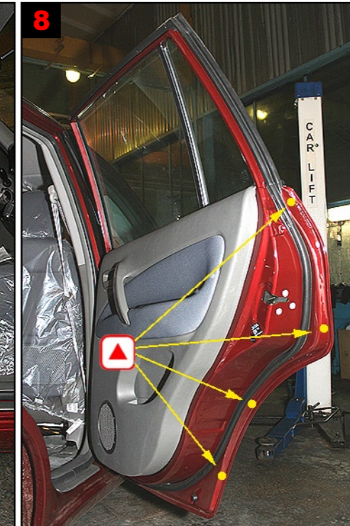
8 Rear door: Treatment via 4 drilled holes.
