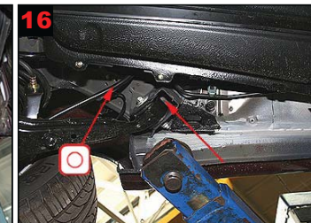
16 Longitudinal member before wheel arch rear and reinforcement: Treat via existing holes and gaps.
