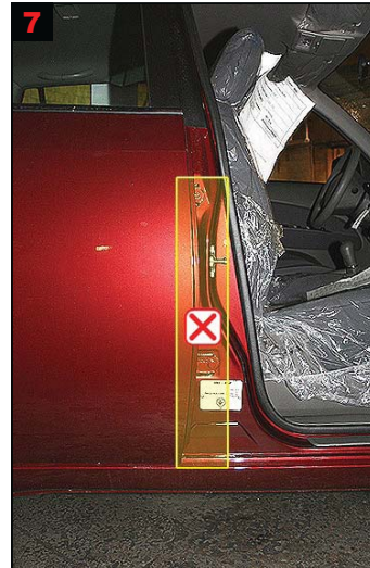
7 B-pillar: No treatment because of safety belt and airbag sensor.
