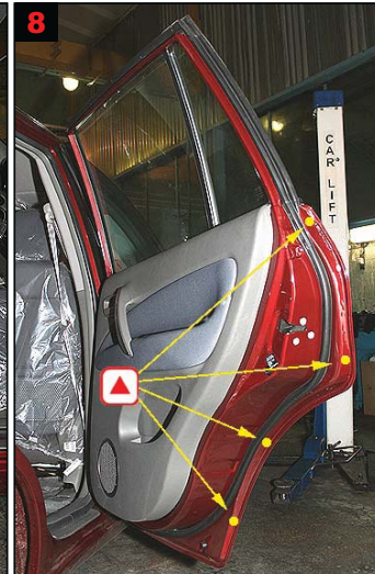
8 Rear door: Treatment via 4 drilled holes.
