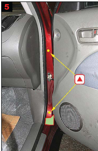
5 A-pillar: Treat via 2 drilled holes. Caution: Foam rubber piece in bottom.
