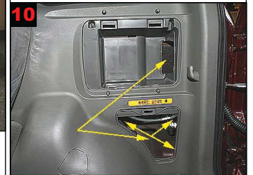
10 Rear wing from boot: Treat from holes in cover plate in boot. Treat in all directions.
