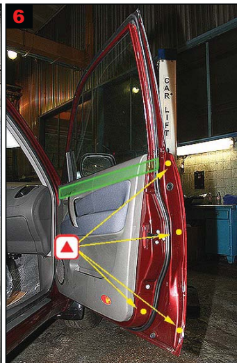
6 Front door: Treatment via 4 drilled holes. Uppermost drill hole for inside reinforcement.
