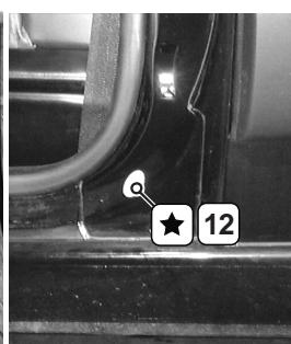
9. longitudinal reinforcement in front wings; right; rear section; remove rubber sealing
