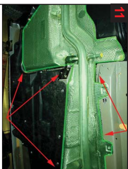
11 Cover plate for exhaust rear. Treat around and behind it where possible.
