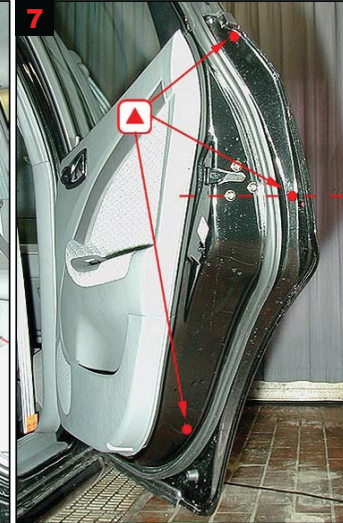
7 Rear door: 3 drill holes for correct treatment. Centre drill hole level with screws for locking device and close to door plate.
