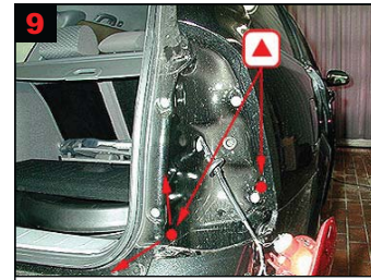
9 Rear wing and rear panel: Remove tail light. Drill 2 holes for correct treatment.
