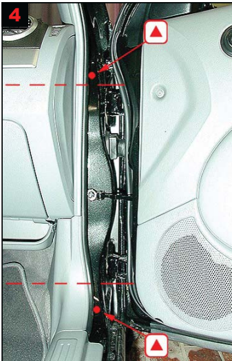
4 A-pillar: Drill 2 holes for correct treatment. Drill level right above and right below door hinges.
