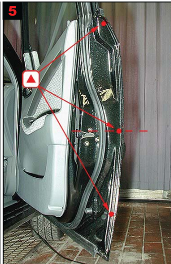
5 Front door: Treat via 3 drilled holes for correct treatment. Centre drill hole level with screws for locking device.
