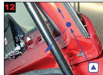
12 Tailgate side: Drill 1 hole for correct treatment.
