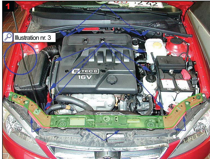
1 Engine compartment: Cowl: Flip plastic plate, treat with caution underneath. Treat along top of longitudinal member, reinforcement for engine suspension right side, under airfilter and battery box, behind spring strut and treat bulb holder and locking plate. See fig. 3 for treatment of top member in front wing.
