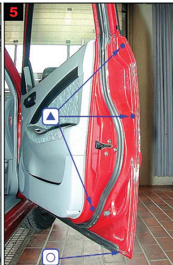
5 Front door: Treat via 3 drilled holes and existing drain hole rear.
