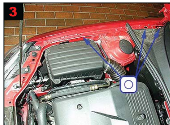
3 Engine compartment - sectional view: Treat top members in front wings via existing holes.
