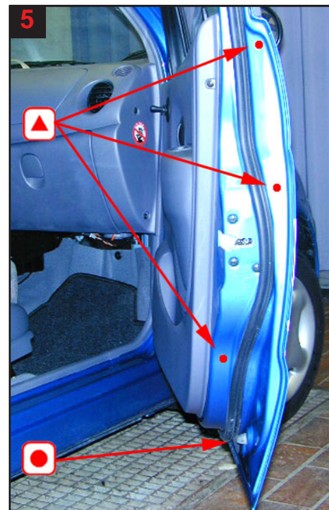
5 Front door: Treat via 3 drilled holes and existing plugged hole.
