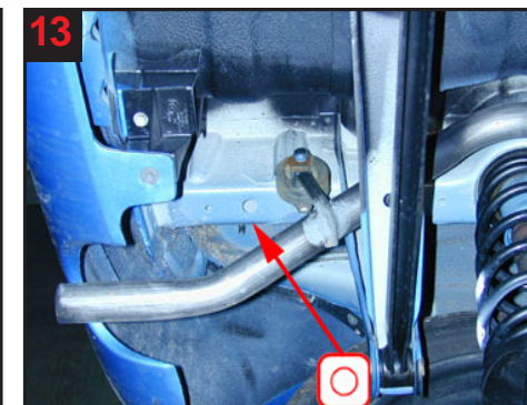
13 Longitudinal member rear: Treat via existing holes.
