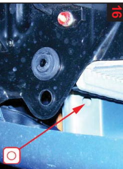
16 Longitudinal members front: Treat via existing holes.
