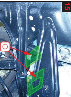
15 Longitudinal member by rack bustling plus reinforcement by engine suspension: Treat via existing holes.
