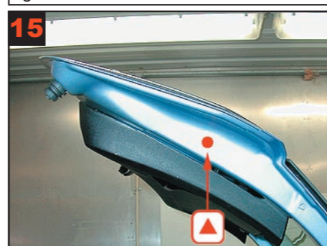
15 Tailgate side: Drill 1 hole for correct treatment. (caution when advancing lance).
