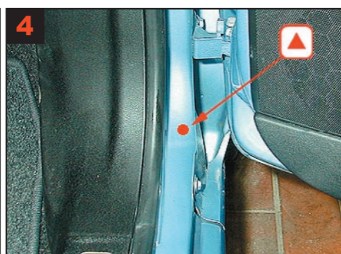
4 A-pillar: Treatment via 1 drilling in panel arch.
