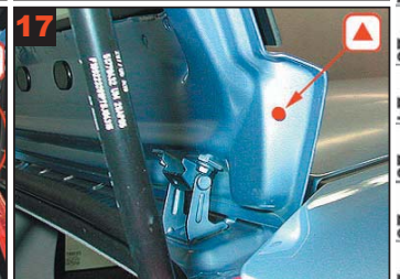
17 Tailgate by roof: Fig: drilling at correct level.
