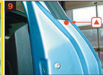
9 Rear door top: Fig: drilling at correct level.
