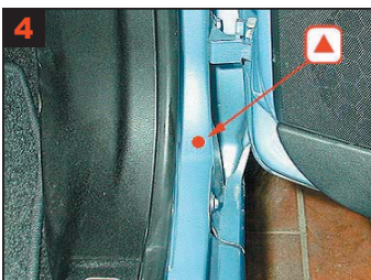
4 A-pillar: Treatment via 1 drilling in panel arch.
