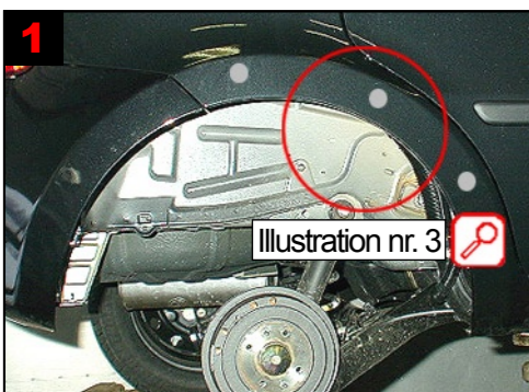
1 Wheel arc rear (wing arc): Remove wheel arch liner. Treat via 3 existing plugged holes. See fig 3 for correct treatment.
