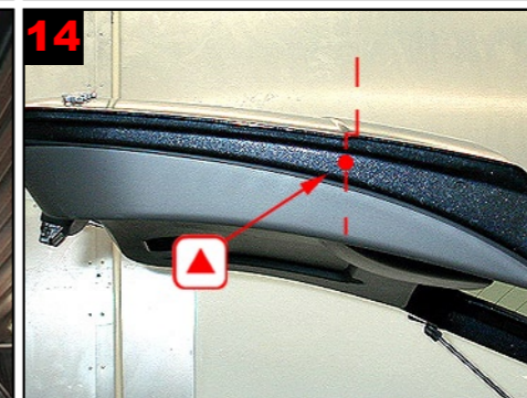
14 Tailgate side: Treat via 1 drilled hole each side. Caution when advancing lance.
