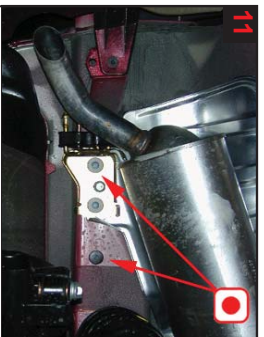
11 Longitudinal member rear. Treat via existing plugged holes.
