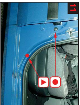
B-pillar: Treat via 1 drilled hole and existing plugged hole.
