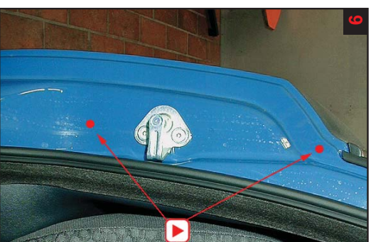
C-pillar: Treat via 2 drilled holes.
