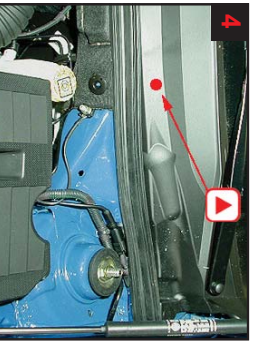
A-pillar: Drill 2 holes for correct treatment.
