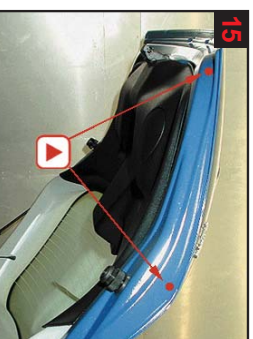
Tailgate side by bumper: Treat via 2 drilled holes - caution when advancing lance.
