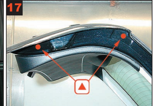
17 Tailgate side: Drill 2 holes for correct treatment. (caution when advancing lance).
