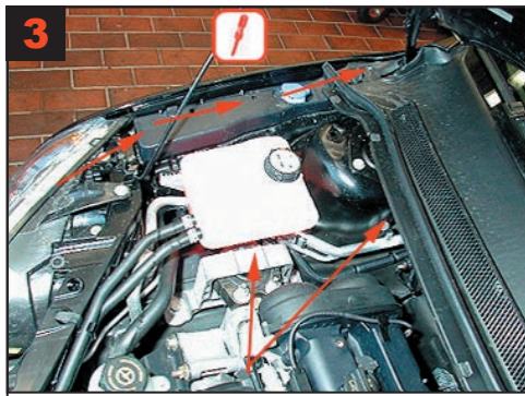
3 Engine compartment sectional view, right side: Flip plastic plate - treat right across. Treatment around hinges for bonnet lid.
