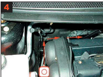
4 Cross member behind engine: Treat via existing holes.
