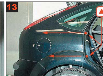
13 C-pillar/rear wing: Drill 2 holes for treatment with lance.
