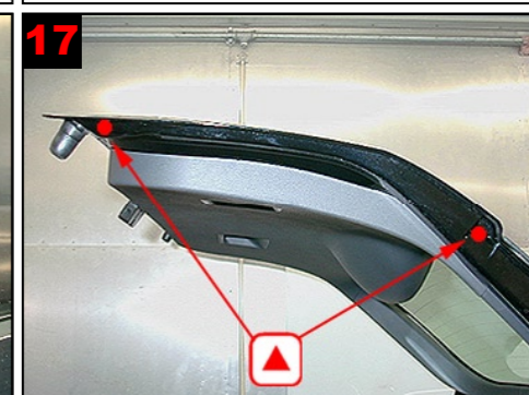
17 Tailgate side: Drill 2 holes for correct treatment. (caution when advancing lance).
