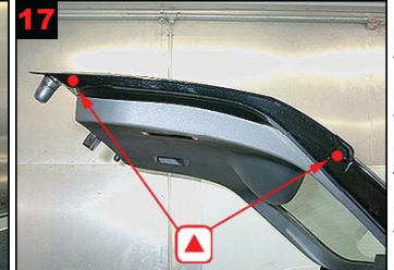
17 Tailgate side: Drill 2 holes for correct treatment. (caution when advancing lance).
