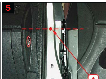
5 A-pillar: Treat via 2 drilled holes. Top drilling level with screw for wing. Lower drilling below door hinge.
