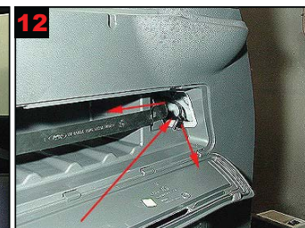
12 Rear wing from boot: Treat via existing lug. Treat in all directions.
