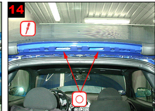
Tailgate by roof: Remove plastic console, treat via existing holes.
