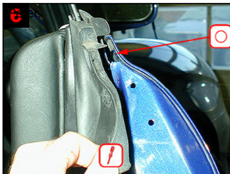
Front door sectional view: Flip rubber plate, treat top member in door via existing gap.
