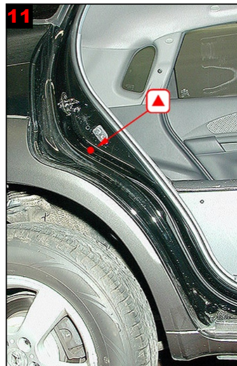
C-pillar/rear wing: Drill 1 hole for part treatment of C-pillar and rear wing. See fig 12.
