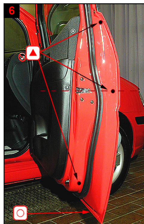
6 Front door: Treat via 3 drilled holes and drain hole. Two uppermost holes is drilled close to door plate.
