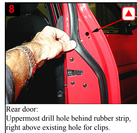
8 Rear door: Uppermost drill hole behind rubber strip, right above existing hole for clips.
