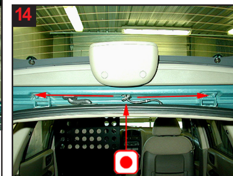
Tailgate by roof: Treat via existing plugged hole.
