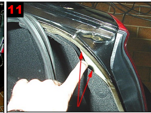
11 Rear wing from boot: Flip lining, treat around tail light.
