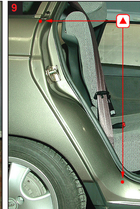
9 C-pillar and rear wing: Drill 2 holes. Uppermost drill hole for part treatment of rear wing.
