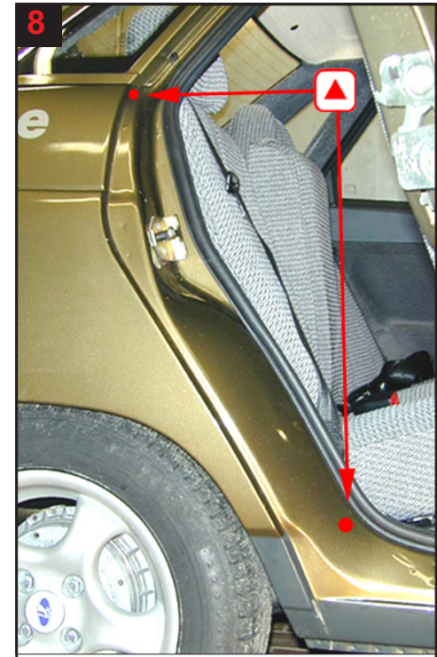
C-pillar: Drill 2 holes. Uppermost drill hole for part treatment of rear wing.
