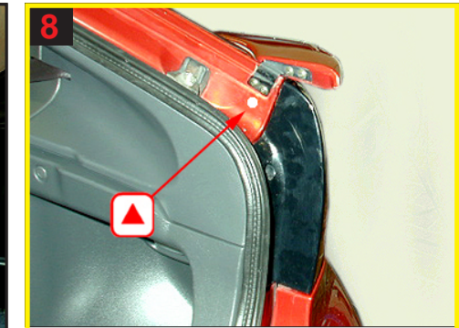
8 Rear wing: Drill 1 hole below mounting for spoiler. Treat with caution.
