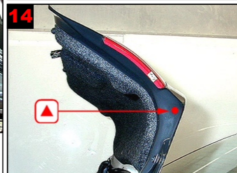
Tailgate side: Treat via 1 drilled hole each side.
