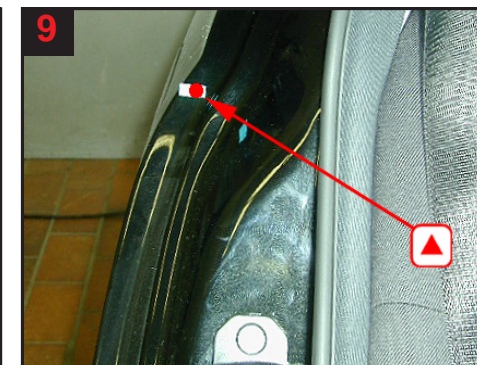
9 C-pillar/rear wing. Drill 1 hole for part treatment of C-pillar and rear wing.
