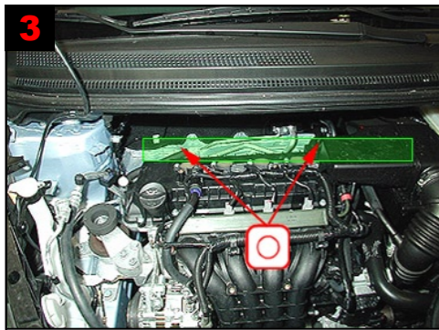
3 Engine compartment - sectional view: Cross member behind engine: Treat via existing holes.
