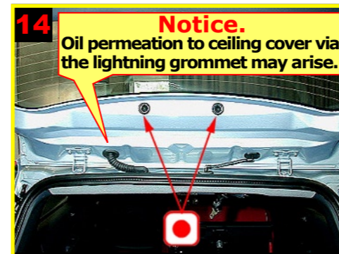
14 Tailgate by roof: Treat via existing plugged holes.
