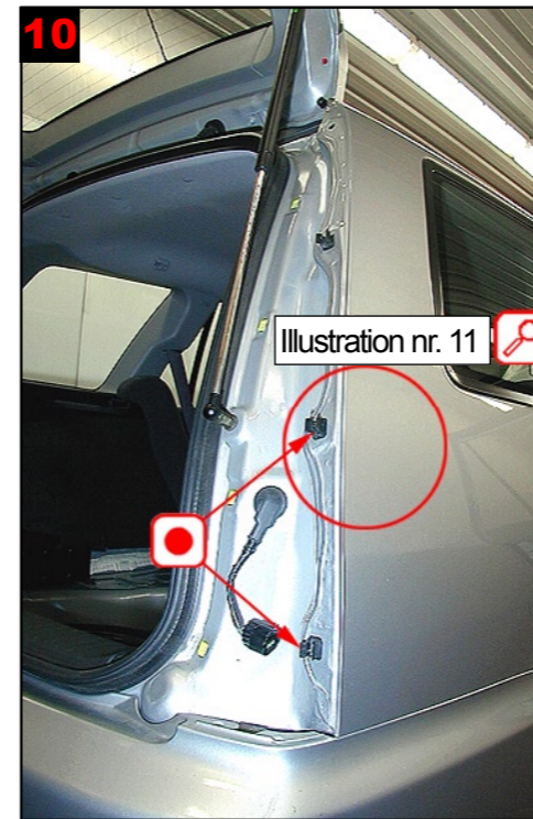
10 Rear wing: Remove tail light. Treat via existing holes for clips.
