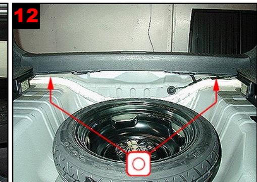
12 Rear panel from boot: Treat via existing holes.
