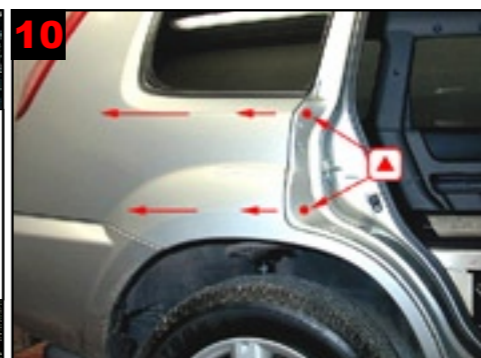
C-pillar/rear wing: Drill 2 holes for correct treatment. Treat with lance.
