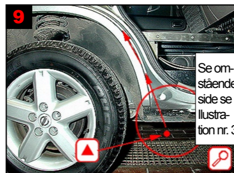
C-pillar/panel: Treat via 1 drilled hole. See the other side of page. See fig 3.
