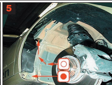
5 Wheel arch front top member: Treat via existing holes and gaps. Treat panel via existing plugged hole.
