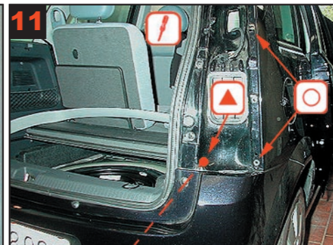
11 C-pillar and rear wing: Remove tail light. Treatment via 1 drill hole and 2 existing holes.
