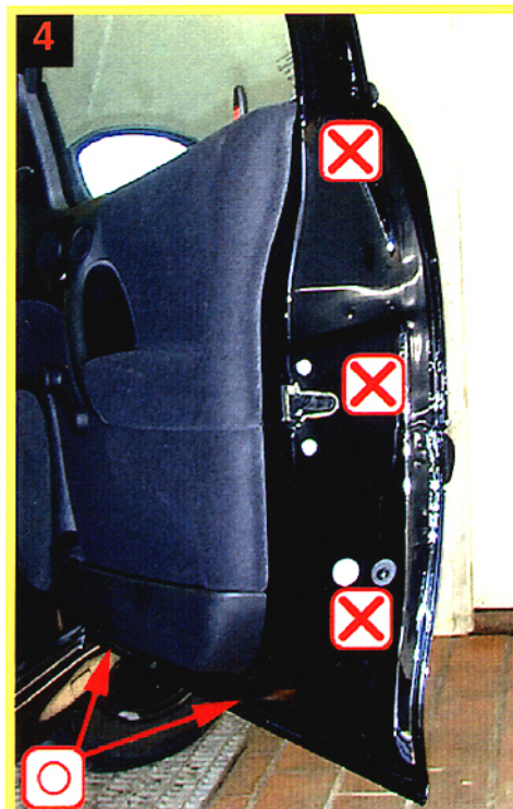
4 Front door. No drilling. Pressure-controlled air bag sensor, treat via drain holes in bottom and existing hole by door stop arm.
