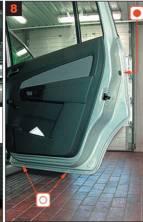
8 Rear door: Treatment via existing plugged hole and drain holes in bottom.
