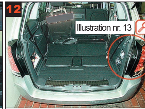
12 Rear wing/rear panel: Treat via 1 drilled hole each side. Fig 13.
