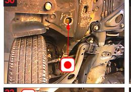
Treat via existing holes from engine compartement. (notce: double member). Treat via existing hole from wheel arch.
